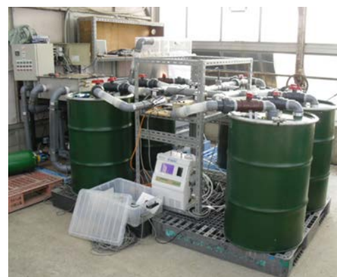
Fig. 2. The CO 2 recovery and application equipment
