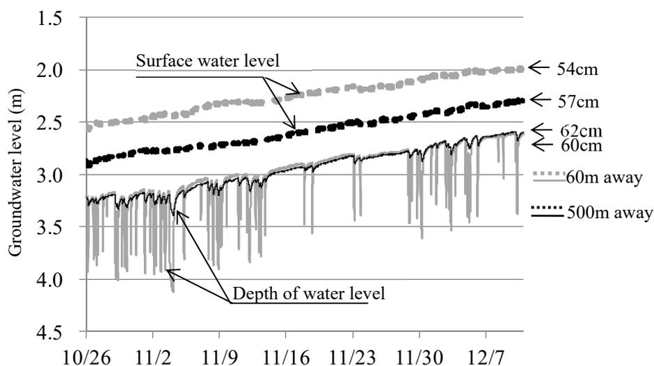
**Fig. 5** Changes in groundwater level during vertical drainage operation
