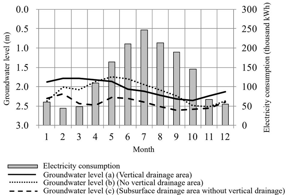
Fig. 3 Changes in groundwater level due to differences in drainage conditions (2012)
