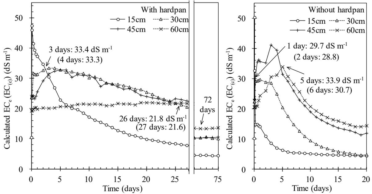
**Fig. 13** Changes in  $EC_e$  during leaching process with 5TE sensor.
