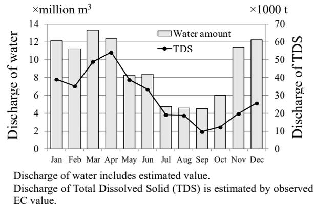
Fig. 4 Discharge and TDS in a collector
