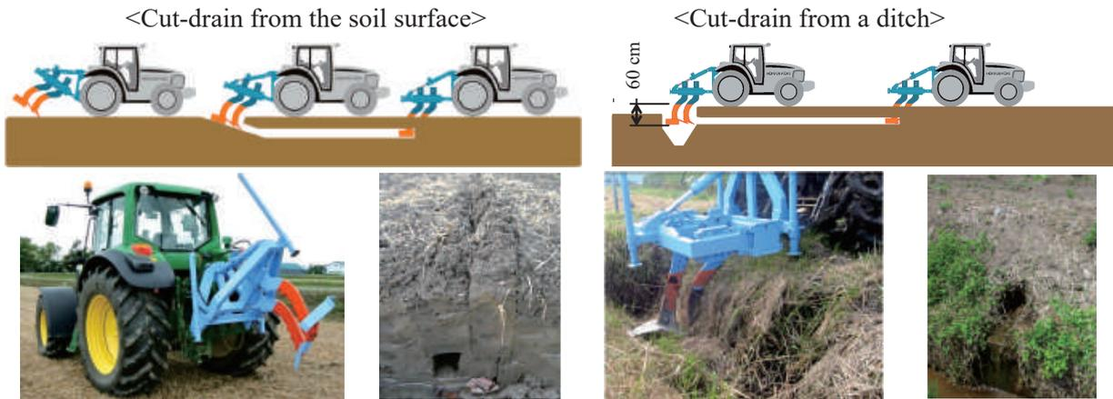
Fig. 2 Drilling method of Cut-drain
