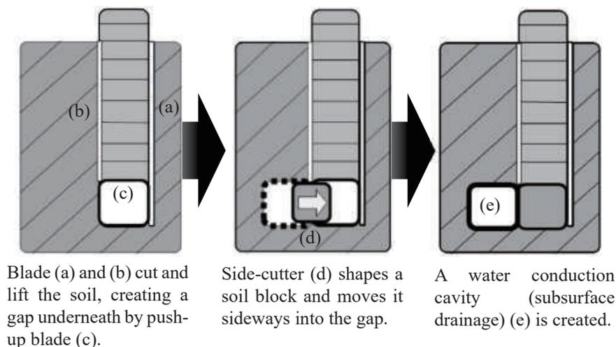
**Fig. 2** Process of making cavity of Cut-drain
