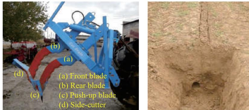
**Fig. 1** Drain-drilling machine and cavity of Cut-drain
