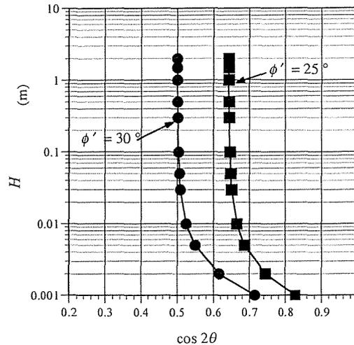
Fig. 7. Relationship between incline of slope  $\theta$  and depth of soil slice  $H$
