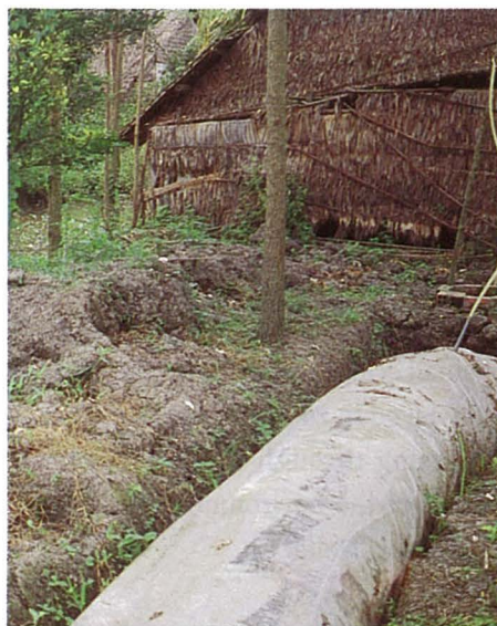
Fig.1. Biodigester of tube type for production of gas using pig feces
