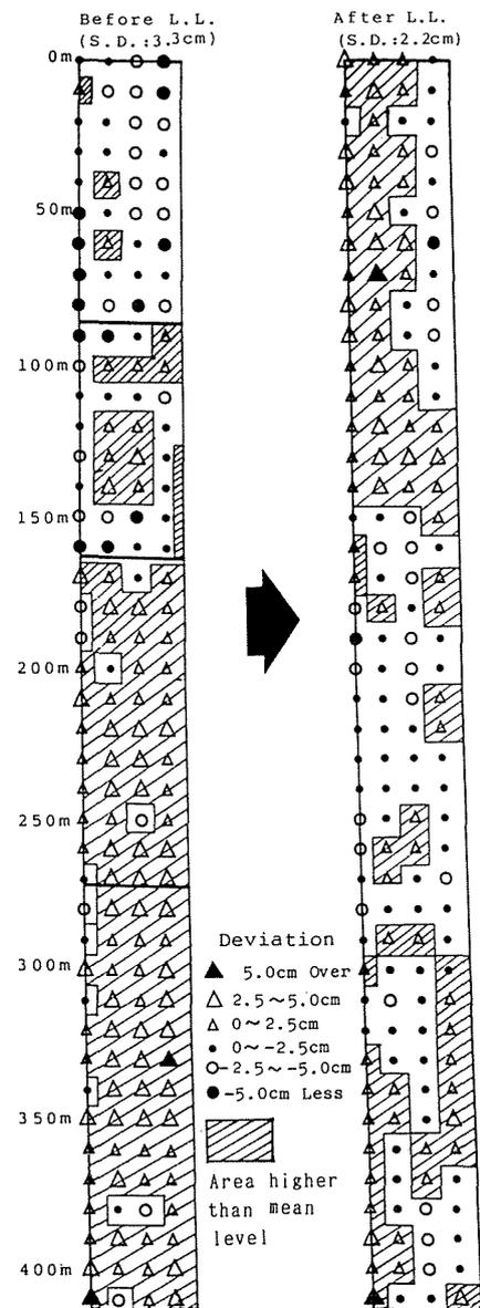
Fig. 3. Field surface level at 10m grid survey points (Experiment 3)
