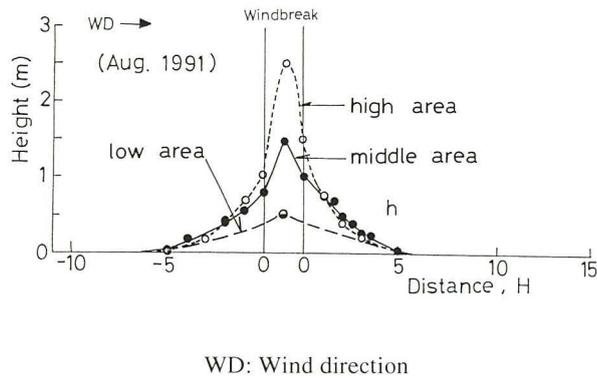
Fig. 1. Variations in sand accumulation induced by single row of tamarisk windbreak in August, 1991
