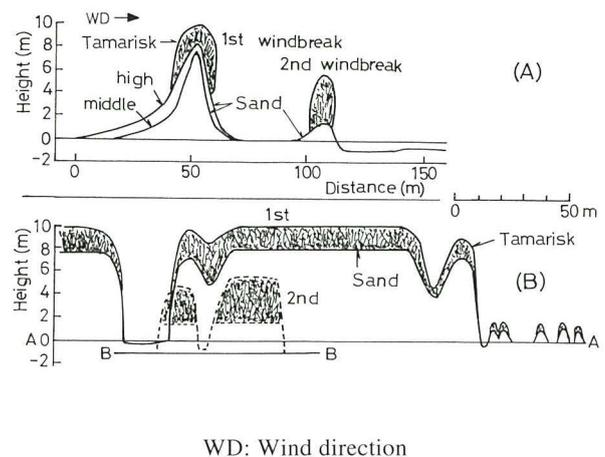
Fig. 2. Schematic diagram of two rows of tamarisk windbreaks and sand accumulation in April, 1992.
